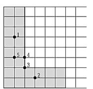
An L-shaped piece, represented by the shaded area on the figure, is cut from a metal plate of uniform thickness. The point that corresponds to the center of mass of the L-shaped piece is A) 1 B) 2 C) 3 D) 4 E) 5
