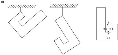
The figure shows a piece of sheet metal suspended in two positions by a string. From the way the metal hangs, you can see that the center of gravity is nearest point A) 1 B) 2 C) 3 D) 4 E) 5
